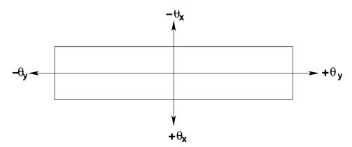
SSM uses one dimensional coded mask. So only the X-coordinate can be calculated for each of the cameras. For the slanted cameras using the calculated values of the x-coordiantes and time difference between the slanted cameras, the Y-coordiantes for the respective cameras can be calculated.
