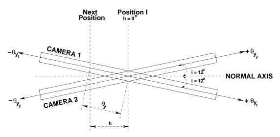
Place the source in position I where difference in  $\theta x = 0$  i.e.  $\theta x_1 - \theta x_2 = 0$  i.e. at position [Ra\_b=Ra\_source + 90°]
